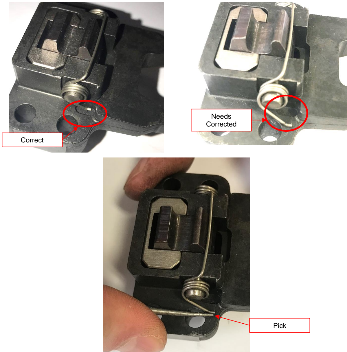
Figure 14 Ensure Corner of Spring is in the Pocket Corner
